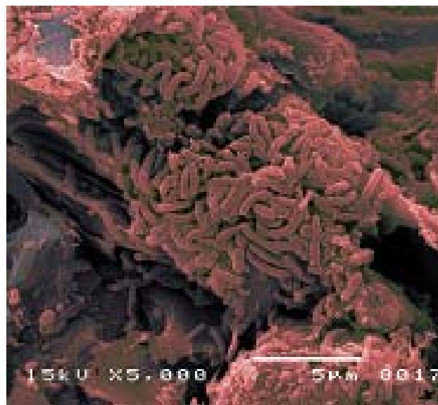
SEM of Geobacter metallireducens producing electricity on an electrode surface, using benzoate as fuel
