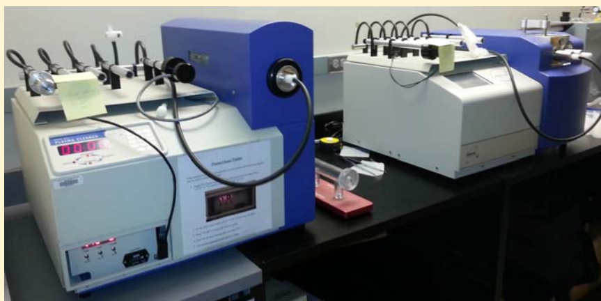
Advanced plasma cleaner for transmission electron microscopy specimens and specimen holders
