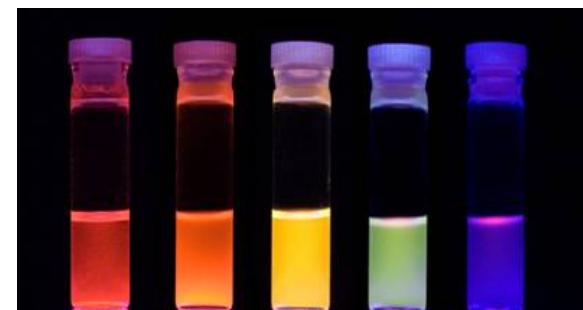
Light Emitting Si-NPs irradiated by a UV source
