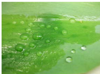
Superhydrophobicity is eliminated by oil fouling
